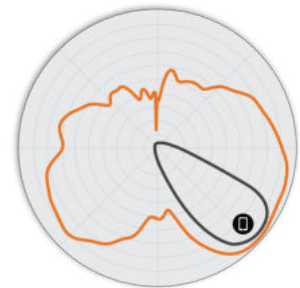
Figure 7. R560 6GHz Elevation Antenna Pattern
